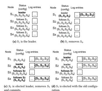
Figure 4. Raft's reconfiguration can violate safety.
