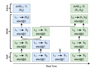
**Figure 14.** Raft to SRaft to Adore refinement.  $L_1 \rightarrow S_1$  denotes a message sent from a leader to a server with the type and logical timestamp of the message indicated below.
