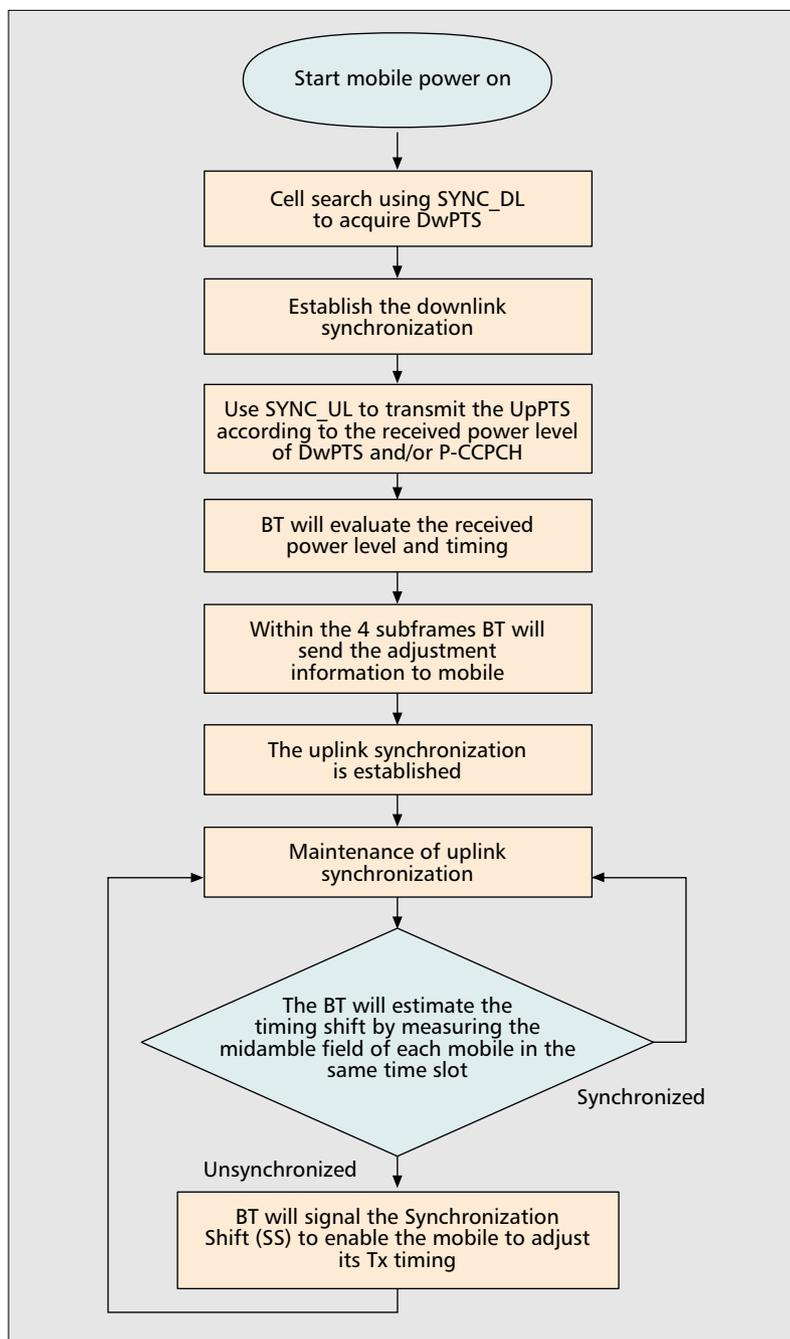
■ Figure 7. A flow chart of the open and closed loop synchronization control adopted in TD-SCDMA for both uplink and downlink, which illustrates that downlink synchronization should be established before uplink synchronization.
