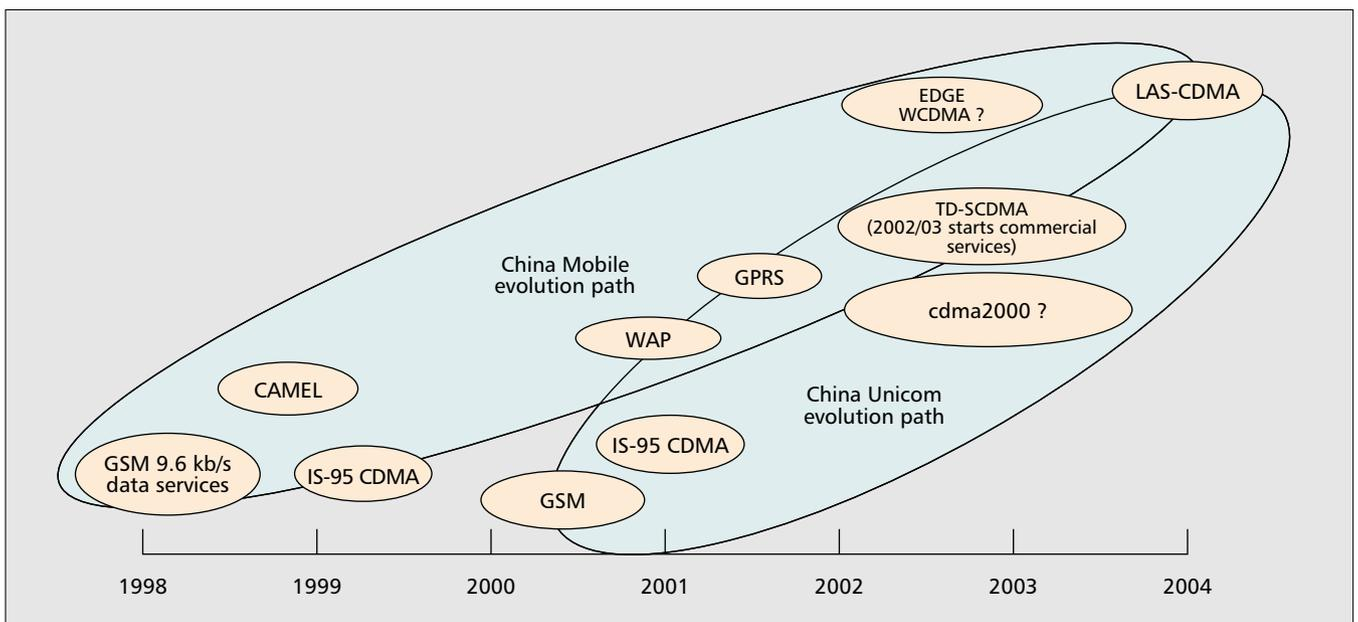
■ Figure 5. The possible evolution paths from 2G to 4G mobile communication systems for China's two current major mobile service providers, China Mobile and China Unicom.
