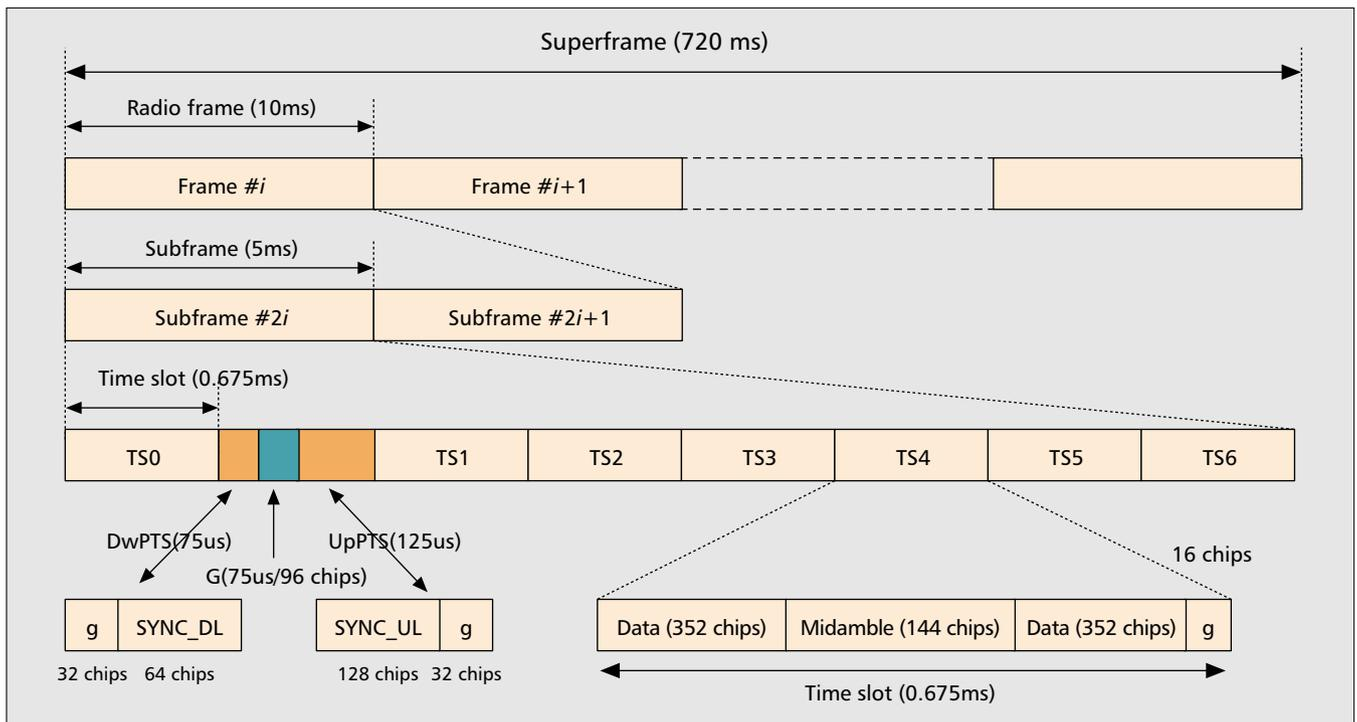
■ **Figure 6.** The four-layered frame hierarchy in TD-SCDMA. TS: time slot; DwPTS: downlink pilot time slot; UpPTS: uplink pilot time slot; G/g: guard period. TS0 is reserved for downlink and TS1 is for uplink only; the rest of the time slots (TS2 to TS6) can form two groups, the first for uplink and the second (which can consist of 1-5 slots) for downlink to suit a particular symmetric/asymmetric traffic requirement.
