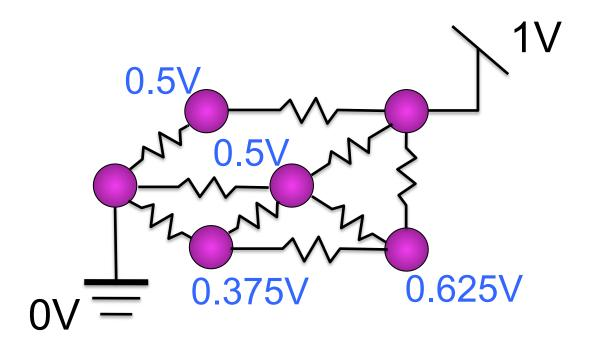
View edges as resistors connecting vertices
