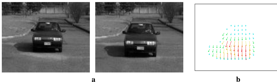
Figure 1.5: Motion as a visual flow. (a) A pair of images in a motion sequence. (b) The optical flow obtained from the pair (all images courtesy of Pierre Kornprobst ,Odyssee Lab, INRIA). Color of vectors encode magnitude. When the magnitude is positive, the field is locally parallel and has dominant local orientation almost everywhere.
