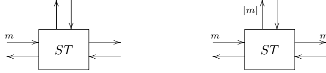
FIGURE 0.4. The ideal functionality modelling a secure channel between two players: upon receiving a message m from one of the two players, it leaks (only) the length |m| and forwards the message to the other player.
