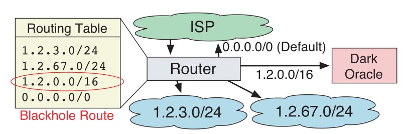
External routing data, internal routing data, host configuration data, and policy device configurations used to construct map of unsued and unreachable addresses
